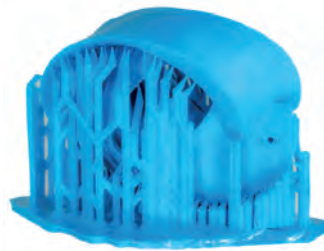
3D printed item showing supporting material
