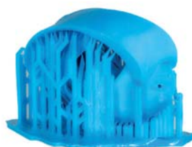
3D printed item showing supporting material
